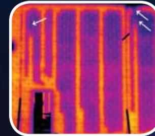
Infrared quality control testing of CMU wall construction.
