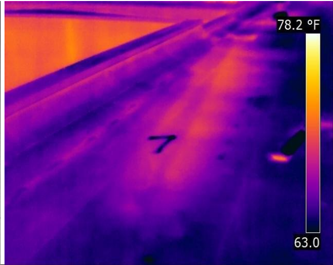
ANOMALY AREA: 7 Date: 8/6/2009 11:39:50 Notes: Suspect area of moisture as indicated.
