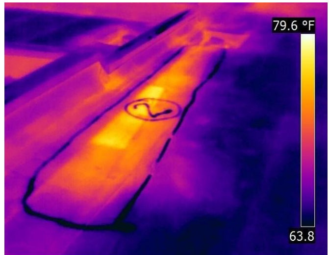
ANOMALY AREA: 2 Date: 8/6/2009 10:55:02 Notes: Suspect area of moisture as indicated.
